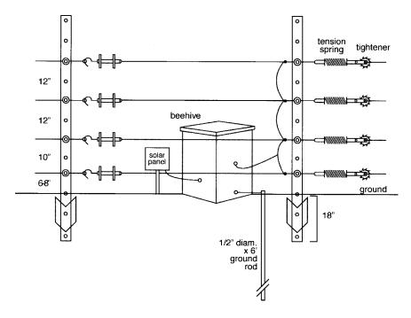
Figure 5: Spacing of electric high-tensile wires and gate, and location of beehive, solar panel and grounding rod behind the fence.
